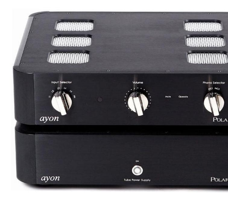
The Polaris is a two-chassis tube preamp design. One piece is the power supply and the other is the preamp. The components are of the exact same size, and while they are a bit on the large side, I was able to fit them into a four-shelf rack rather easily. Dimensions are 21x18x5 inches for each unit and they weigh in at 72.6 lbs for the pair.
